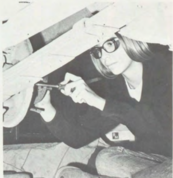
Studying the technical aspects of brake adjustment, Billy Jo Kramer replaces a faulty brake lining.
